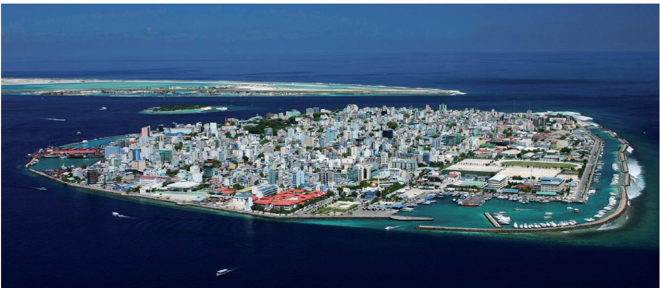
The overpopulated Island of Male, capital of the Maldives, is protected by dikes. Two raised artificial islands were built 2 km away by filling the lagoon with tons of sand and dead coral. They accommodate buildings, a hospital, a mosque and an airport.
