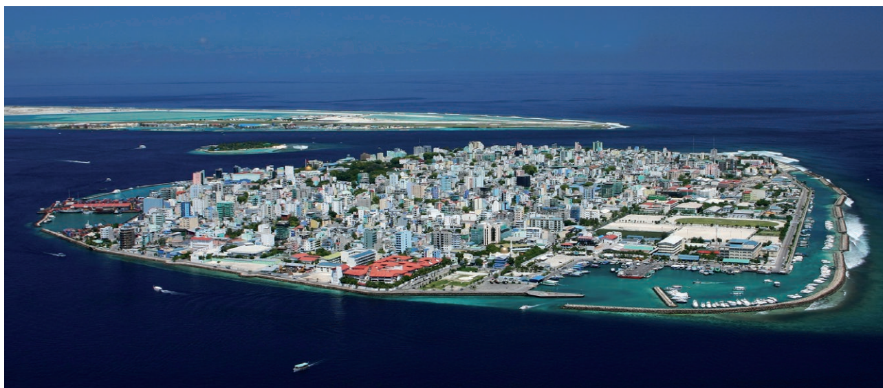
The overpopulated Island of Male, capital of the Maldives, is protected by dikes. Two raised artificial islands were built 2 km away by filling the lagoon with tons of sand and dead coral. They accommodate buildings, a hospital, a mosque and an airport.
